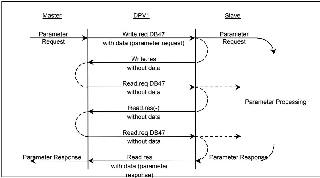
Fig.14 Telegram sequence via DPV1
