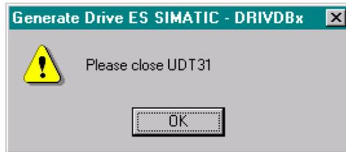
If library DRVDPS7 is not installed in the standard installation path for libraries (...\\s7libs), or it does not contain UDT31 (SLOT\_UDT), the following window appears and the data block(s) is (are) not generated. The program is then terminated.
