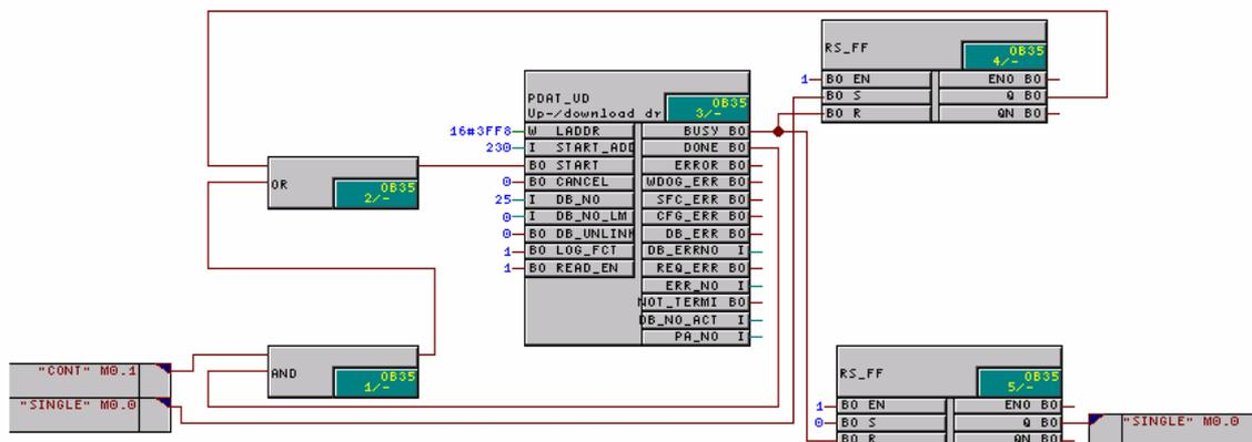
**Structure of the parameter job (example of complete DB transfer)**
