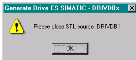
After the source has been generated, the program checks whether the block folder of the selected CPU contains UDT31 (SLOT\_UDT). If not, it is copied to the folder from library DRVDPS7.
