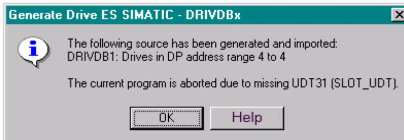
When the generation and copying processes are finished, a window appears showing the free data block number assigned to the new sources.
