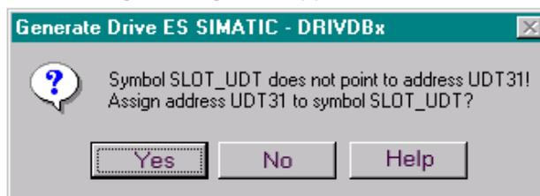
If both UDT31 and the SLOT\_UDT symbol are already assigned in the project, you must correct the assignment or delete the entries from the symbol table. The following message box is displayed to remind you:
