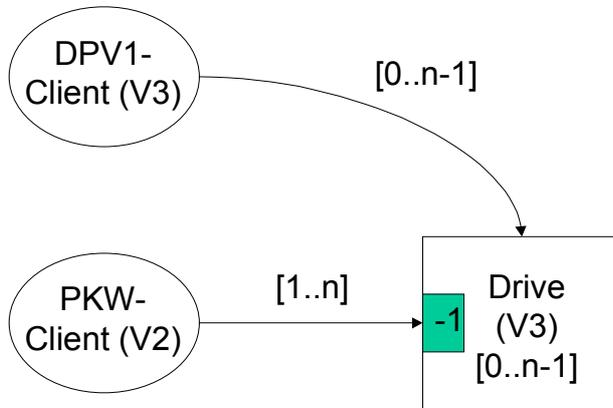
Fig. 65 Interface characteristics of the devices according to profile version 3
