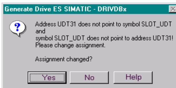
If the SLOT\_UDT symbol is assigned to address UDT31 in the symbol table after the above message is displayed, a message indicating that UDT31 will be overwritten after the symbol table has been checked again:
