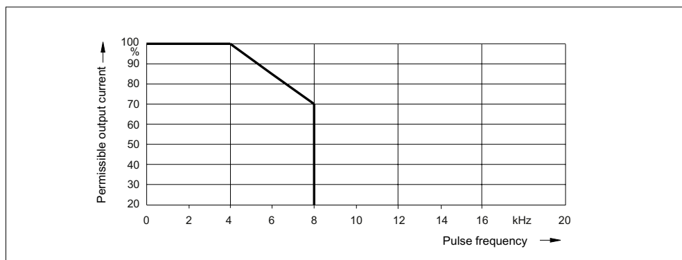
Figure 3-27 Frame size FSF: Output current as a function of the pulse frequency
