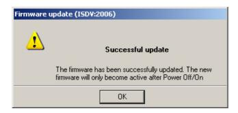
4. After the firmware update, switch off and on the 24 VDC supply power. Only then is the new version shown in the version overview.
