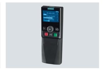
A handheld version of the IOP can be ordered for mobile use. In addition to the IOP, this includes a housing with rechargeable batteries, charging unit and RS232 interface cable. The charging unit is supplied with connector adapters for Europe, the US and UK. When the batteries are fully charged, the operating time is up to 8 hours.
