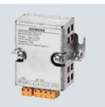
The Safe Brake Relay allows the Power Module to be safely connected to an electromechanical motor brake, allowing the brake to be directly and safely controlled by the Control Unit in accordance with EN 954-1 Safety Category 3 and IEC 61508 SIL 2.
