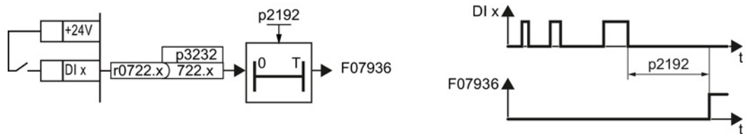
Figure 8-33 Function plan and time response of load-interruption monitoring
