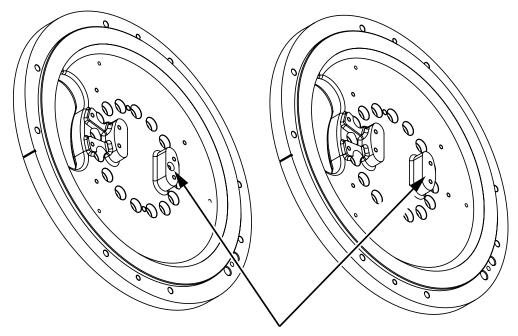
There are two different designs of the swing plate, inside the base. One of the designs has an air release hole and the other does not.
