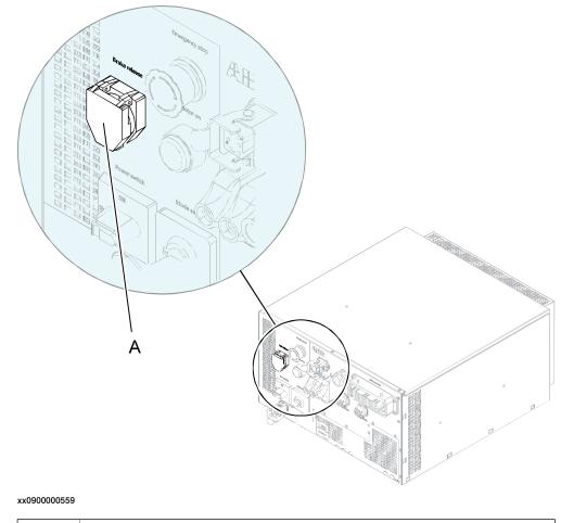
Brake release button (beneath the cover)
